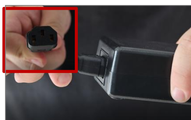
6. Connect the power cord to the scanner and plug it into a power outlet
