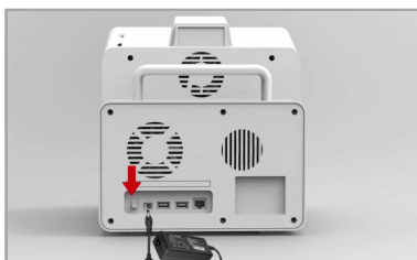
7. Turn on the power switch in the back of the instrument
